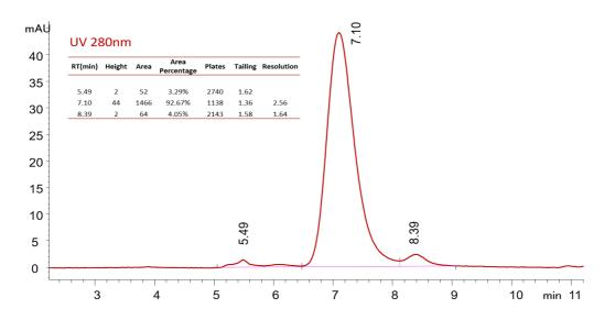
Column: Sepax SRT SEC-500, 5μm, 500 Å, 7.8×300mm (P/N: <u>215500-7830</u>); Mobile Phase: 2.0X DPBS pH 7.5; Flow rate: 1 mL/min; System: HPLC; Column Temperature: 25 °C; Detection: UV 280 nm; Sample: AAV5 2.22x1013GC/mL in DPBS with 0.001% F68; Injection volume: 50 μL
